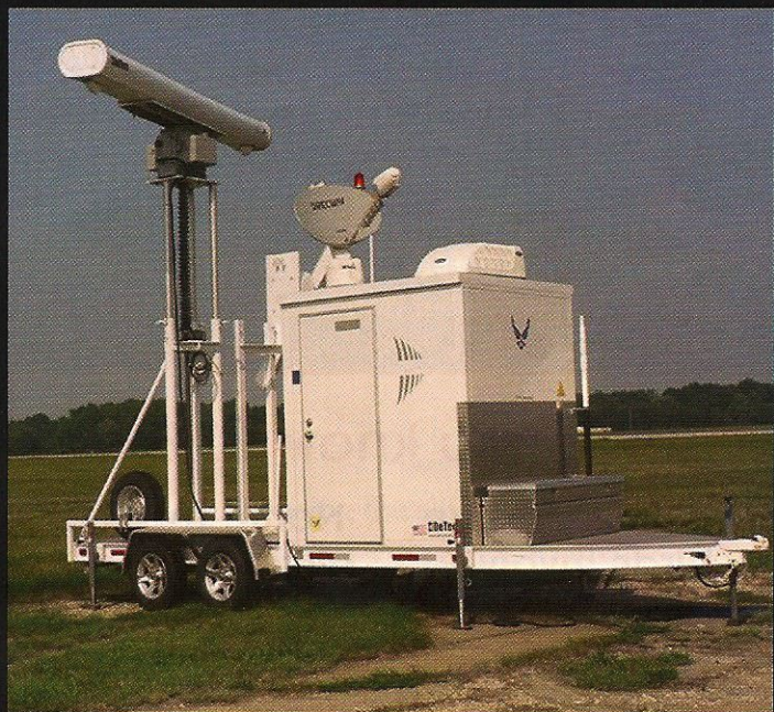
Top and above: Bird radar at Dover AFB.
